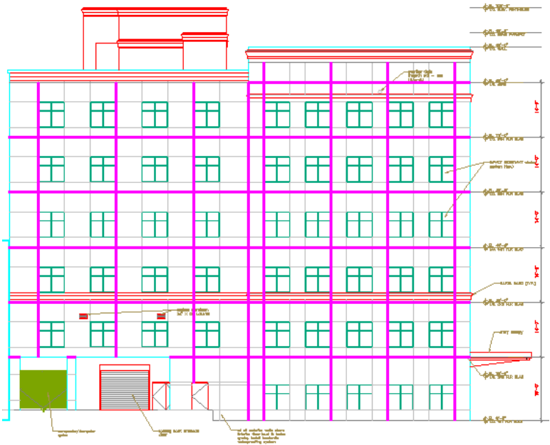
Figure 4.9, Designed Expansion Joints (Magenta) for East Facade
