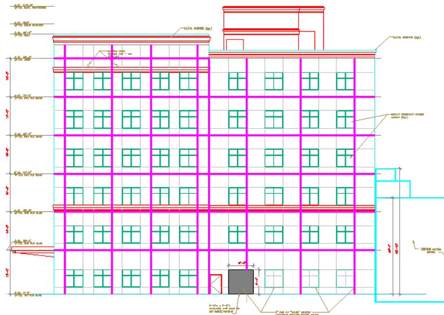
Figure 4.10, Designed Expansion Joints (Magenta) for West Facade
