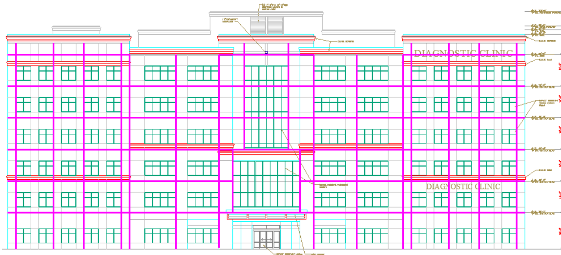
Figure 4.7, Designed Expansion Joints (Magenta) for North Façade
