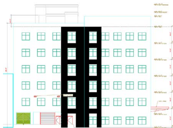
Figure 2.2, Lateral Force Resisting Elements at East Side Source: Oliver, Glidden, Spina & Partners
